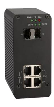
Xentino **TI940** is an Industrial 6-port Gigabit PoE Switch, the switch equips with 4-port **10/100/1000M RJ45** PoE+ and 2-port Gigabit SFP open slot. The 4 PoE+ ports are IEEE 802.3at compliant which supports up to **30W** per port.
