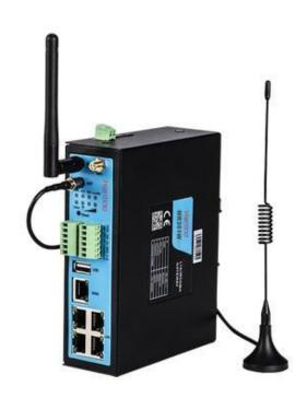
MR351W is an OpenWrt based Linux OS industrial IoT gateway, which provides C/C++, Python programmable embedded environment for IoT developers and programmers to implement their industrial applications in a flexible and easy way.
