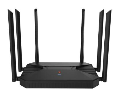
RL207 is an 11ac standard dual band indoor 4G wireless router support VPN. Comply with IEEE 802.11ac/b/g/n MIMO standard, the data rate up to 1200Mbps, more than 80 end users can access into it with SIM card slot, build in QUECTEL LTE module. It supports FDD-LTE/TDD-LTE for worldwide use with 150Mbps (CAT4) downlink speed. Besides that, there are 3\*10/100Mbps WAN/LAN ports, automatically switch to WAN Ethernet if 4G network existed.
