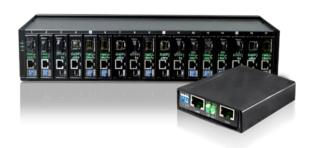
Xentino VX100-DC VDSL2 Extender Modem Router High-speed, Long Reach Ethernet Extender with one RJ-45 Ethernet port and one RJ-45 VDSL port. It is a bridge mode modem to extend Ethernet over single-pair phone line. Transfers 100Mbps of symmetric data rate over the existing copper wires. It also supports both symmetric and asymmetric transmission, and can reach up to 100/100 Mbps bandwidth (line rate) within 300M or 10/10 Mbps (line rate) for 1Km long range connections. DC powered.
