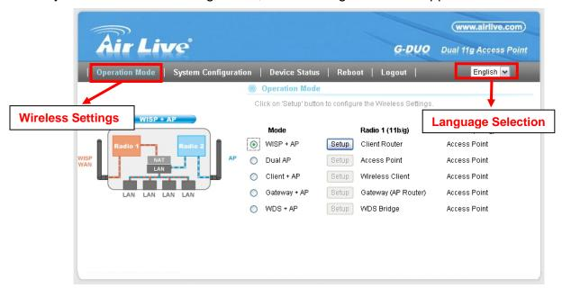
Wireless Settings: The G.DUO's wireless settings are different between wireless modes. Only functions that are applicable to the wireless mode will show to simplify configuration. For this reason, the first step to configure the G.DUO is to select the wireless mode. The router mode specific functions are also in this
