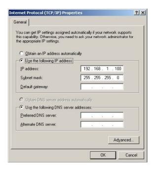
Fig. 1-1, Assign IP as 192.168.1.100/255.255.255.0 onto your computer
