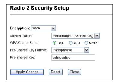
■ Encryption Type: There are two encryption types TKIP and CCMP (AES). While CCMP provides better security than TKIP, some wireless client stations may not be equipped with the hardware to support it. You can select Mixed to allow TKIP clients and CCMP clients to connect to the Access Point at the same time.
