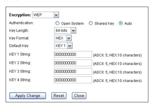
■ Select one of the WEP key for wireless network: There are total of 4 possible keys for WEP encryption. You need to choose which key will be used for encryption. All wireless devices on the same network have to use the same settings. We recommend using WEP Key 1 as in default setting.
