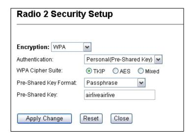
■ Encryption Type: There are two encryption types TKIP and CCMP (AES). While
