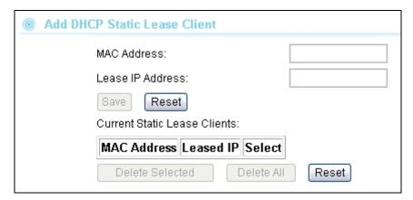
If you want to lock IP address to a MAC address, you should add DHCP clients to the "Static Lease Client". Up to 40 entries can be entered. Below is the procedure for adding an entry:
