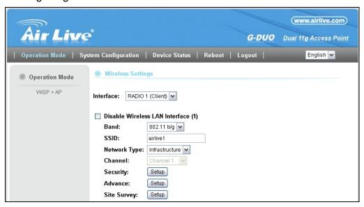
**Step2:** Click on "Site Survey" Setup button. The following screen should appear with results of available APs in the area.
