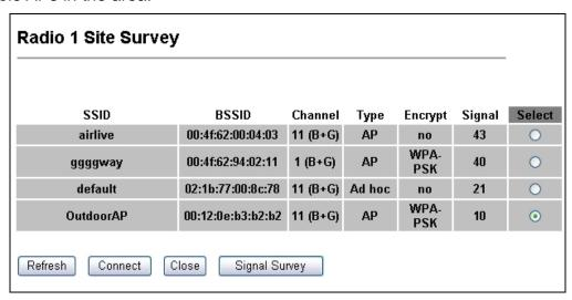
**Step2:** Now select "Outdoor AP" on the list, then press "Signal Survey". Adjust your antenna until the signal level is at the highest.
