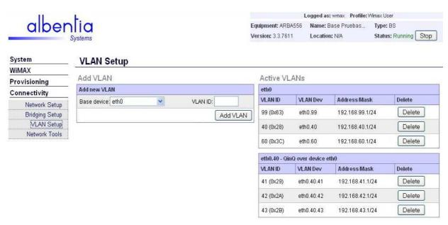
Figure 74 - "VLAN Setup" menu
