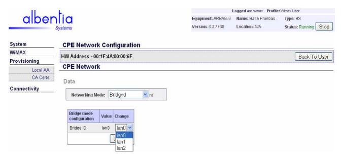
Figure 61 - CPE Network Configuration - Bridging mode
